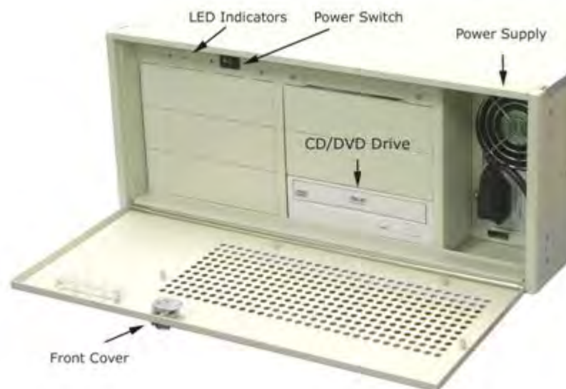
Figure 3-1: 4901-Front view, shown with cover open.
