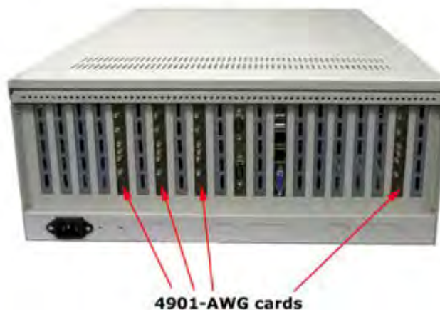
Figure 3-2: 4901-Rear View showing four 4901-AWGx cards as well as serial, Ethernet, USB and monitor connectors.
